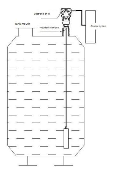
Note:Please use a wrench to screw the instrument base during installation, and do not screw the meter head directly.
